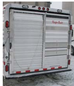
Opt – “Roll-Up Rear Door ILO Standard ½ Slide” unit above is shown on an 8’ wide trailer with Optional Rear “Recessed Back-Up Lights” (pair)
