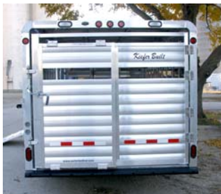
Std – “Rear Gate Full-Swing ½ Slide w/2” Rubber Rollers and Nylon Pads w/Slam Latch” unit above is shown on an 8’ wide trailer with Optional Rear “Recessed Back-Up Lights” (pair)
