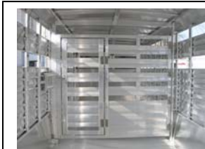
Std – “Center Divider Gate w/ Walk-thru Door w/ Slam Latch” in 6’ 6” Height, 7’ wide trailer, with #2 sidewall configuration, closed.
