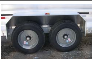
Opt – Various Axle Options available – contact factory for additional information Std. Extruded Fender and Cat Walk Shown for 7’ wide Trailers
